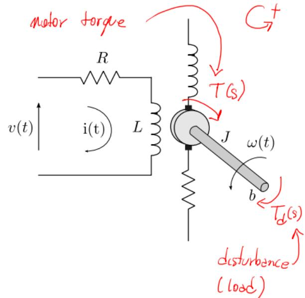
$$T(s) = (Js^2 + bs)\theta(s) + T_d \rightarrow \theta(s) = \frac{I(s)k_i - T_d}{Js^2 + bs} \rightarrow \omega(s) = \frac{I(s)k_i - T_d}{Js + b}$$
