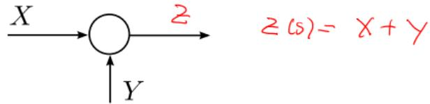
A block diagram showing a circular block with two inputs. The top input is labeled  $X$  and the bottom input is labeled  $Y$ . The output signal  $Z$  exits the block from the right.
