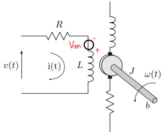
→ Back electromagnetic force voltage
