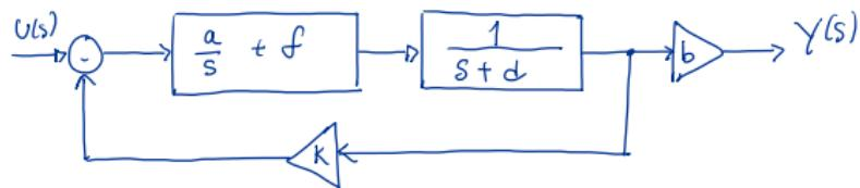
$$\frac{Y(s)}{U(s)} = \frac{\left(\frac{a}{s} + f\right)\left(\frac{1}{s+d}\right)}{1 + K\left(\frac{a}{s} + f\right)\left(\frac{1}{s+d}\right)} b = b \frac{a + fs}{s^2 + ds + K(a + fs)} \quad (4)$$
