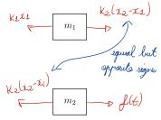
Find the differential equations to model the behaviour of the system shown.
